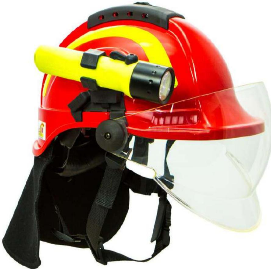
Helmet TYTAN type HOT 101.04 is a state-of-the-art helmet intended for use for wildland firefighting (grassland fires, forest fires) and during technical and road rescue. The innovative structure of the helmet's shell is made from fibreglass-reinforced polyamide using injection technology. This guarantees high mechanical strength and thermal resistance. It is a multi-purpose, light and ventilated helmet with excellent basic equipment.
